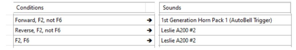
Not pressing F6 a multi-chime horn is used in forward direction; the Leslie A200 #2 (copied in to a Sound Slot from the Sound Library) is used in reverse direction. Pressing F6 sets the horn to the Leslie A200 in either direction.
